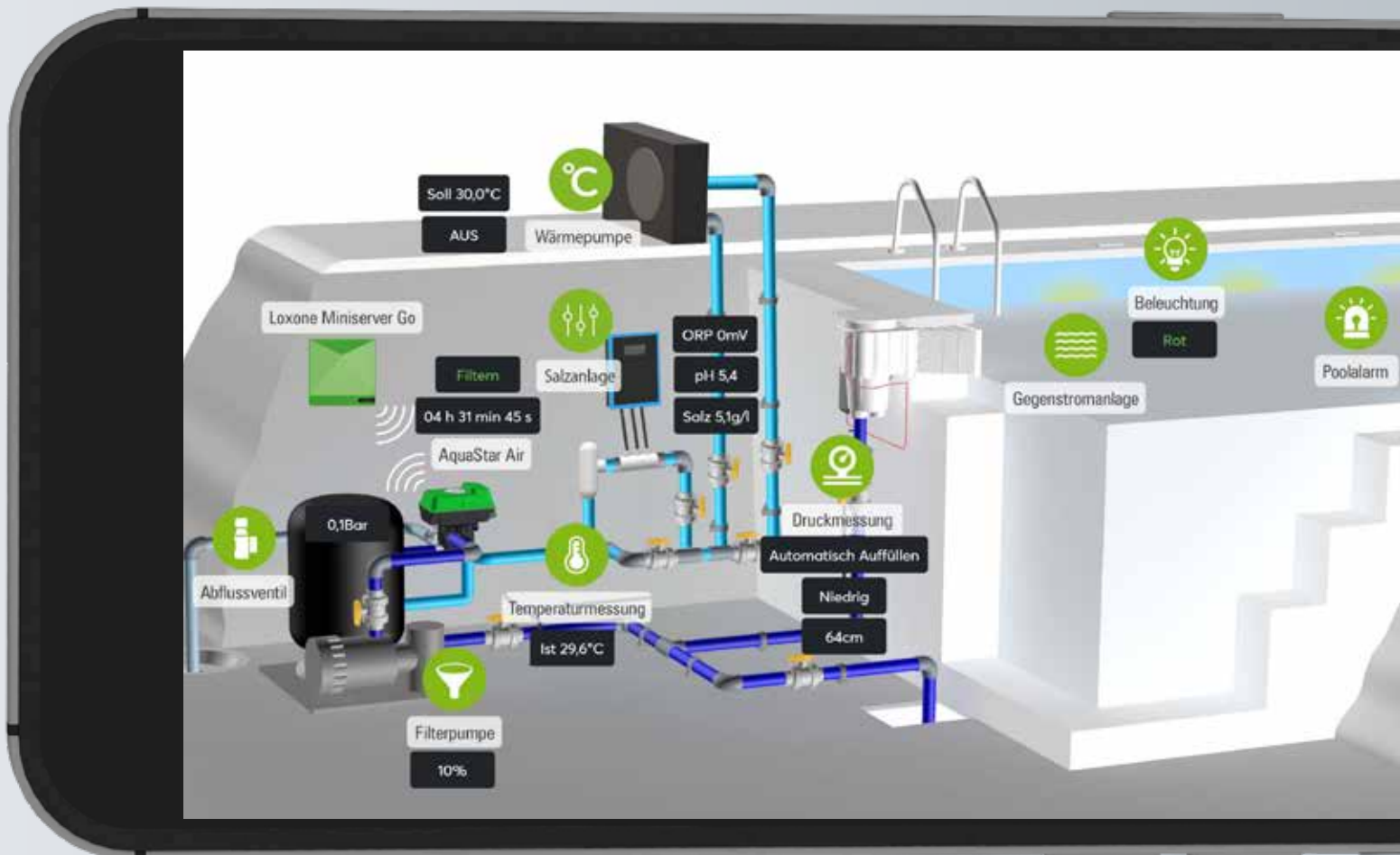
The system diagram in the app provides a clear display of all pool settings and values, such as pH level, redox potential, and salt content. The values can be adjusted directly through the diagram.
