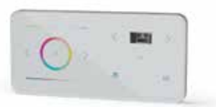
The remote control unit Link Touch RGB is specifically designed for RGB lights. Link Touch adjustable white only works with white lights.
